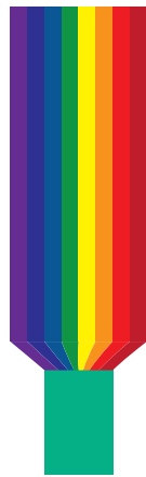
CWDM Transmission (Up to 18 Signals)
